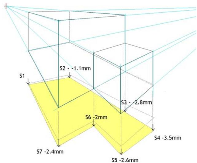
The movement between S2 and S4 for example, is uniform along the length of the wall. Using "L/360" as the limiting tensile stress, we see (below) theoretical permissible movement of 7.2mm, against actual movement at the end of August of 3.5mm. A drop of 2.4mm over a length of 10.45mtrs from the front corner of the house to the rear corner of the extension is hardly subsidence.
