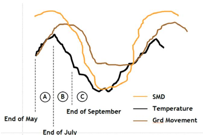
Ground movement continues even as the temperature begins to drop (interval 'B'), and the energy to drive this has to be the tree. No other element (wind, relative humidity or solar radiation) accounts for this relationship.
